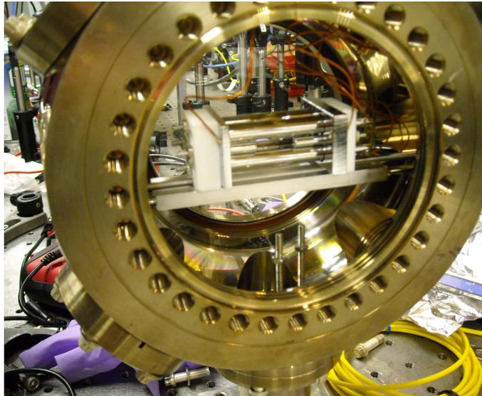
Figure 1.2. Assembled trap housed inside an octagonal vacuum chamber.
