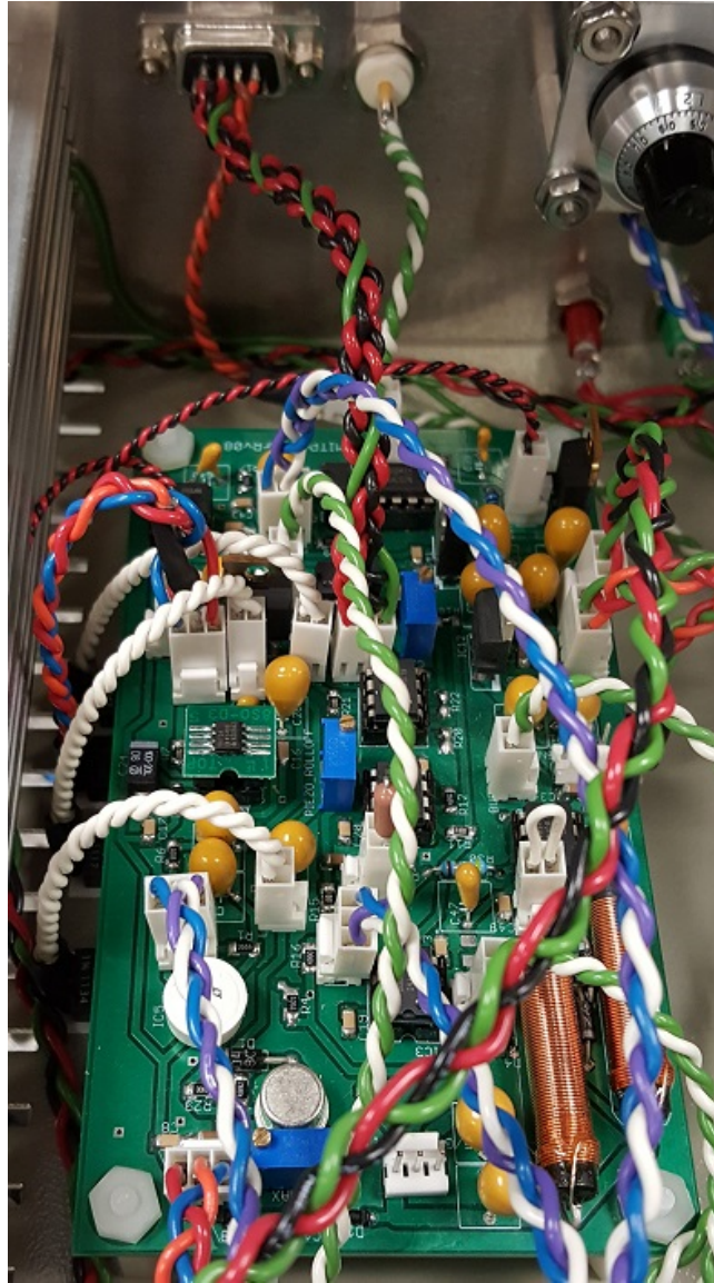
Figure 2.11. Picture of an assembled current driver in an ECDL electronics system. All wiring is 22 AWG.
