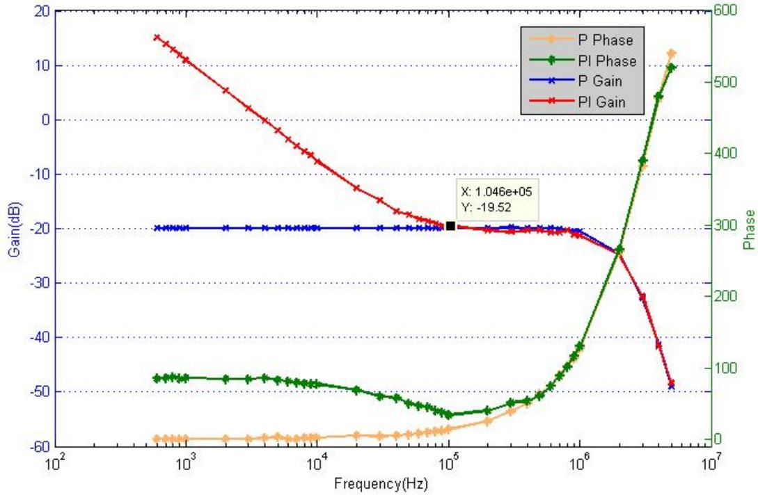
Figure 6.2. PID circuit performance. The blue line represents the P gain, and the red line represents PI gain, corresponding to the left axis. The yellow line represents the phase of the circuit only when P stage is working. The green line represents the phase of PI both working.
