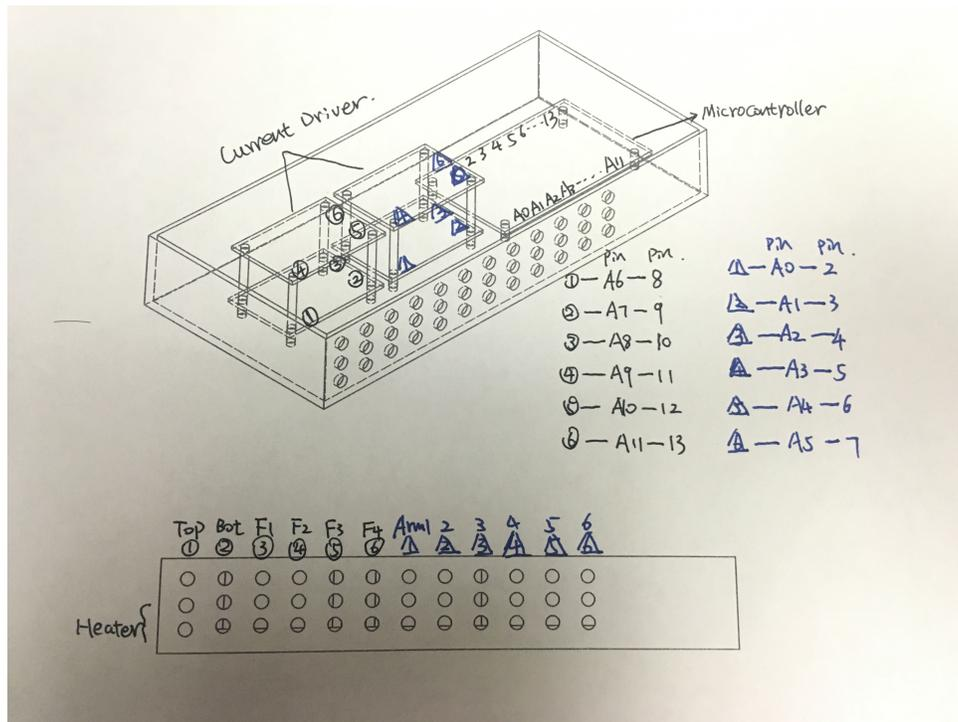
Figure B.4. Schematic of the wire connections of current driver electronic and the microcontroller.
