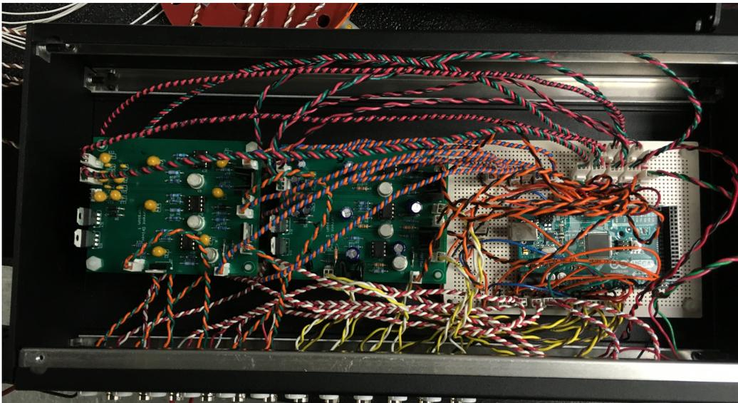
Figure B.1. Photo of the instrucional amplifier electronic.
