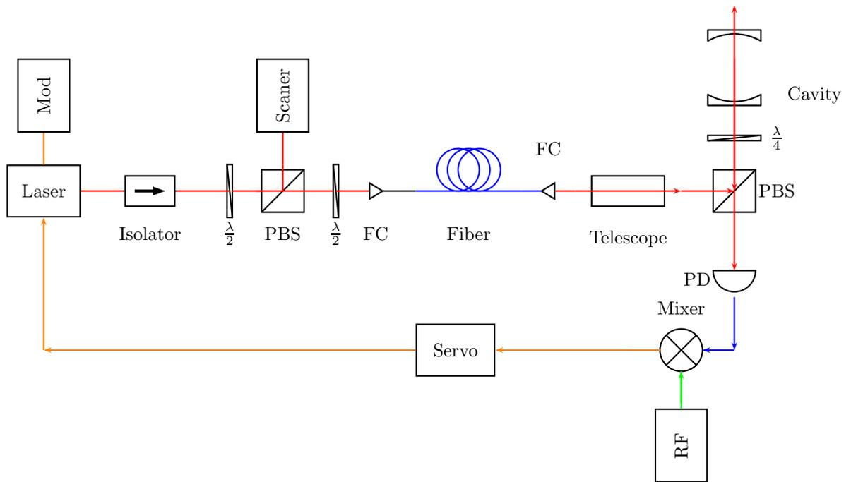
Figure 2.5. This figure shows the layout of the experiment setup. The red line represents laser beam, other color lines are signal paths. The signal going to the laser controls its frequency.
