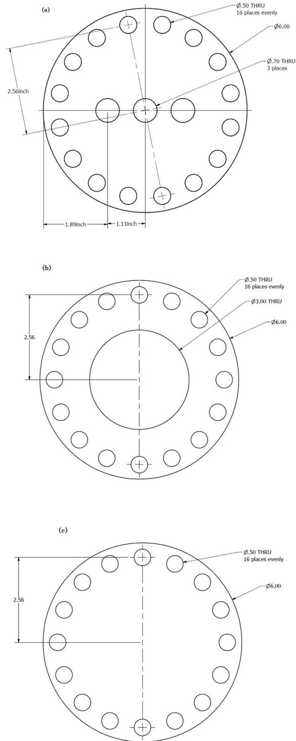
Figure 4.2. Design of the heater for the vacuum chamber's faces. (a) is the heater for the viewport, the three holes in the middle are used for guiding laser into the cavity. (b) is the heater for the top face (reducer), the middle holes are used for installing ion pump. (c) is the heater for the bottom.
