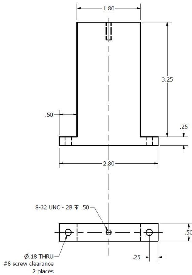
Figure A.1. Design of the stand used to support the cavity in the chamber.
