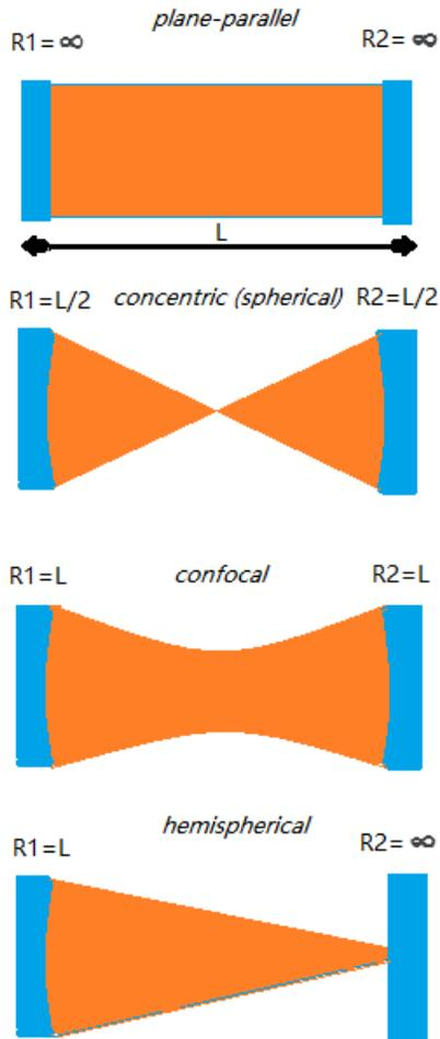
Figure 3.2. Four kinds of optical cavities, with mirrors of various curvature, showing the radiation pattern inside each cavity
