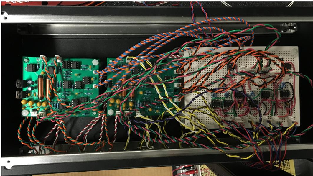
Figure B.3. Photo of the current driver electronic and the microcontroller.
