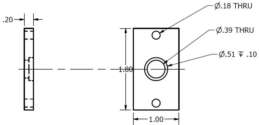
Figure A.3. Design of the mirror holder attached to the baseplate and hold the cavity mirrors.
