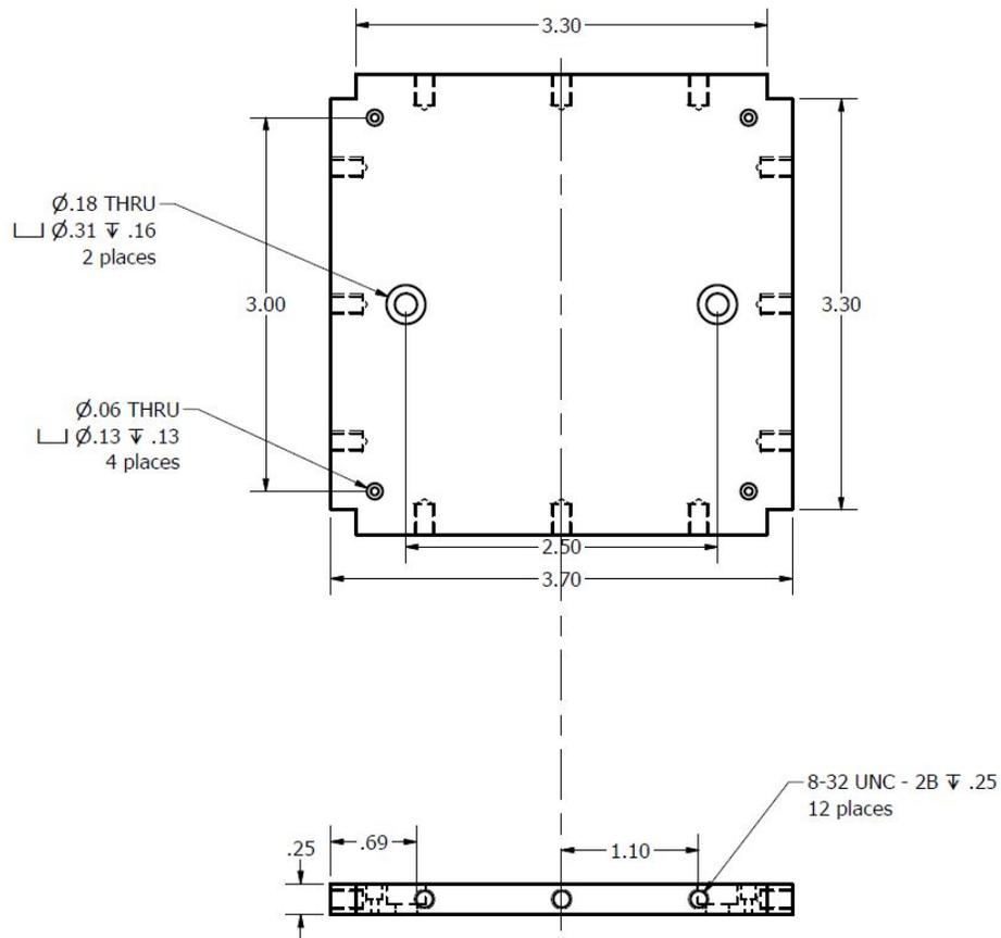
Figure A.2. Design of the baseplate connected to the stand and used to attach the mirror holders.
