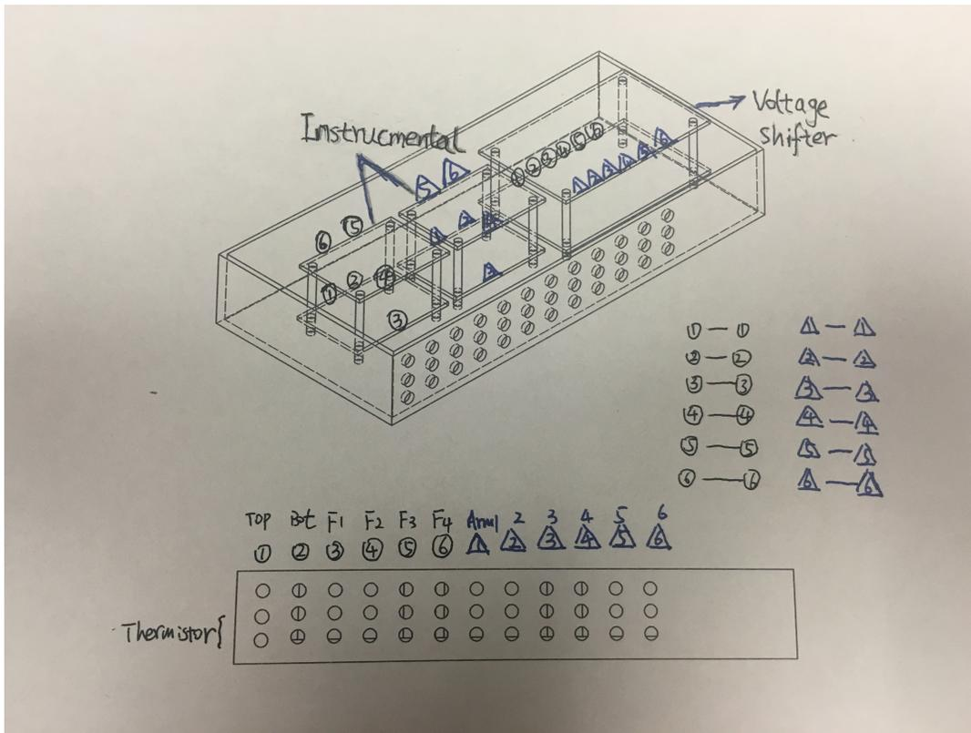
Figure B.2. Schematic of the wire connections of instrumental amplifier electronic.
