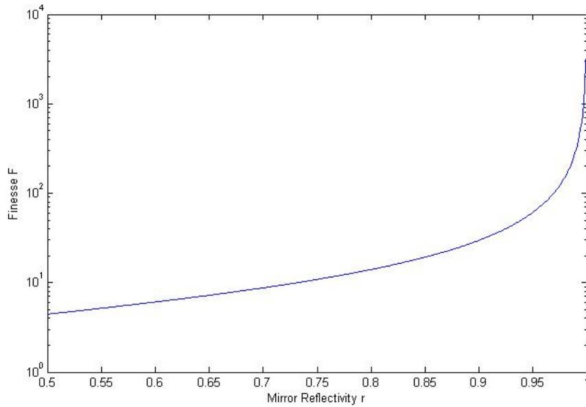
Figure 3.4. Finesse as a function of reflectivity. Very high finesse factors require highly reflective mirrors.
