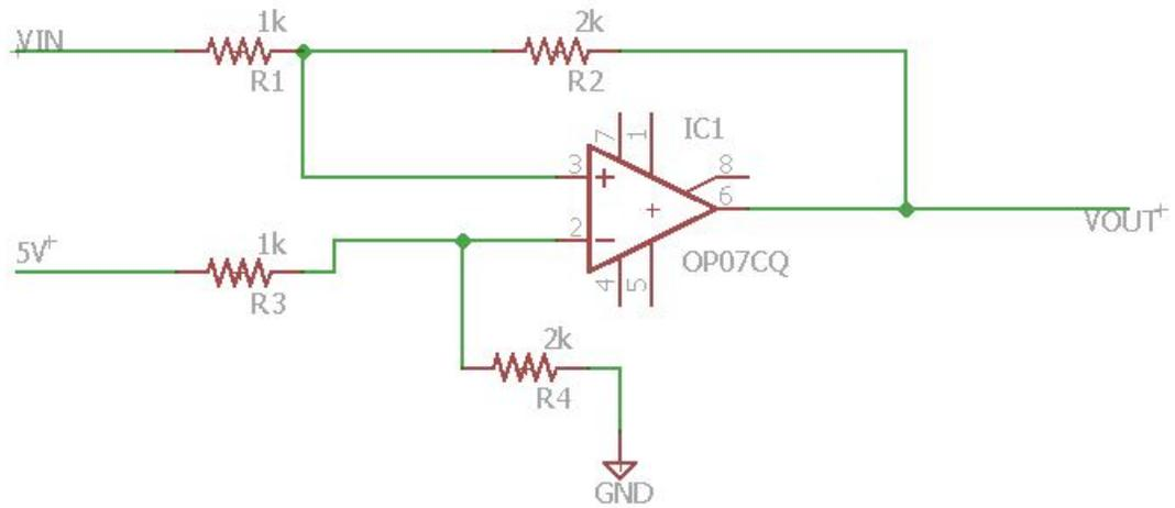
Figure 4.4. Schematic of an adder. IC1 is op amplifier OP07. One input is the error signal, the other input is 5V.
