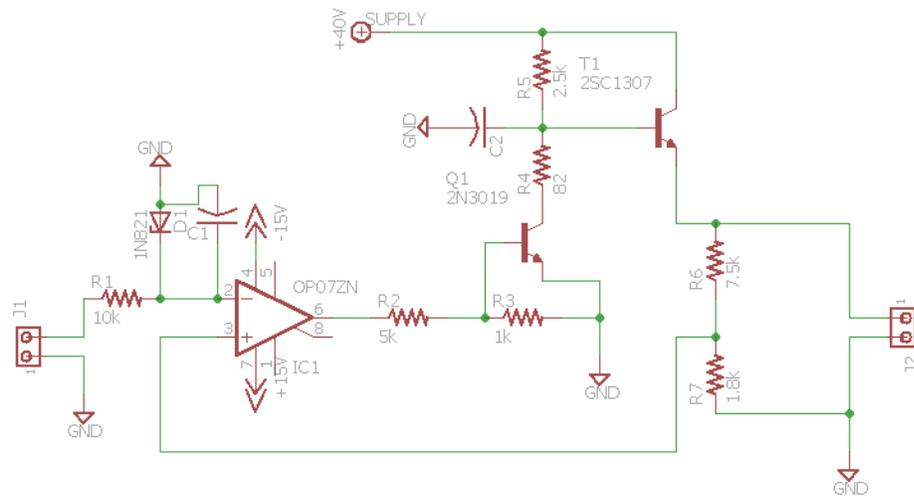
Figure 4.3. Schematic of the current driver to control the heaters. The operational amplifier IC1 is OP07. The transistor Q1 and T1 are 2N3019 and 2N6043 separately. D1 is a diode.
