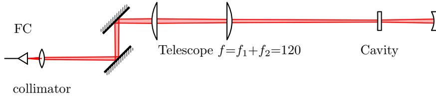
Figure 5.1. Mode-Matching setup. This telescope is made of two identical convex lens with  $f = 60\text{mm}$ . The two parallel mirrors in this figure are used for aligning beam to hit the center of the first mirror of the cavity.
