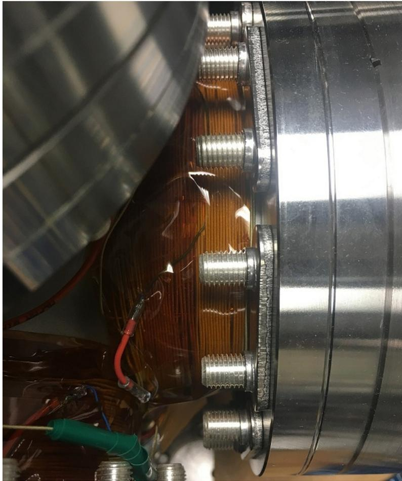
Figure 4.1. Photo of the heater around the arm of the vacuum chamber. The yellow wire under the tape is the heater. The blue one is the thermistor connected to the red wire. In each arm we use four thermistors to measure temperature.
