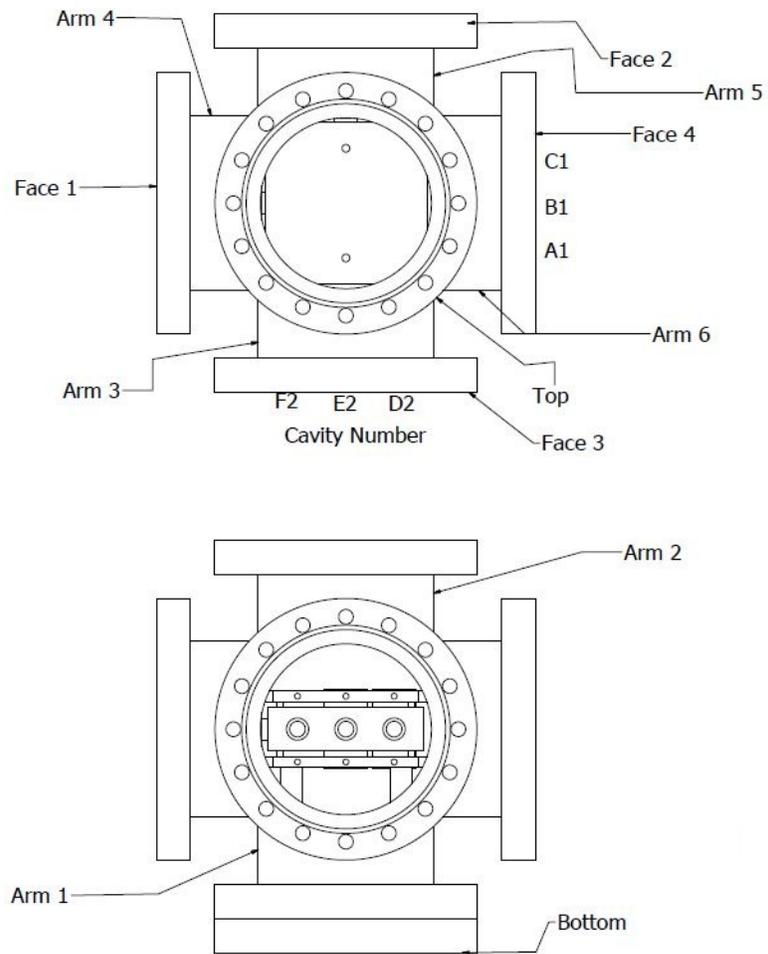
Figure B.5. Schematic of chamber's arm number and face number.
