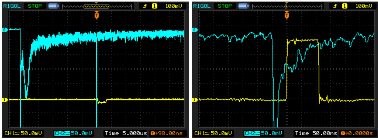
(a) PMT signal, \mu\text{sec} scale, showing fluorescence from the ablation plume which may have complicated structure and persist for up to 10's of nsec.
