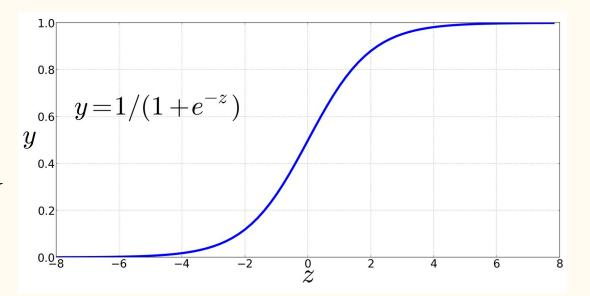
x axis = sum of weights times inputs y axis = output value of neuron
