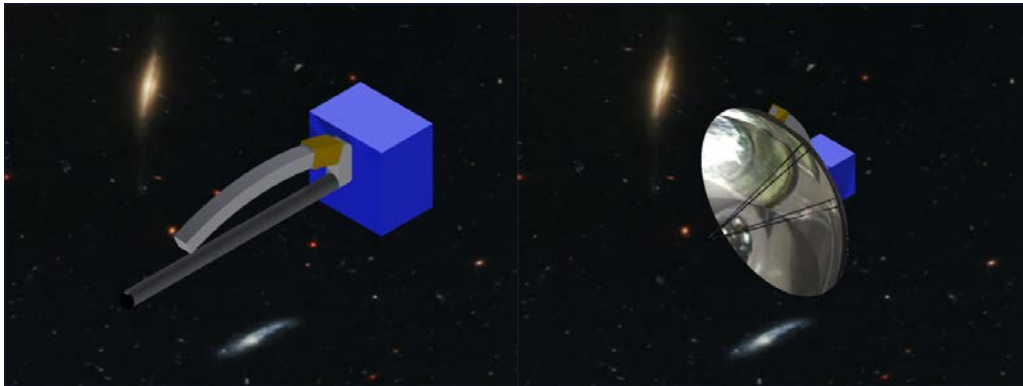
Figure 1. Before and After Deployment (Write Head in Gold Color Moves along the Curved Arm, while the Curved Arm Rotates about the Center Axis)
