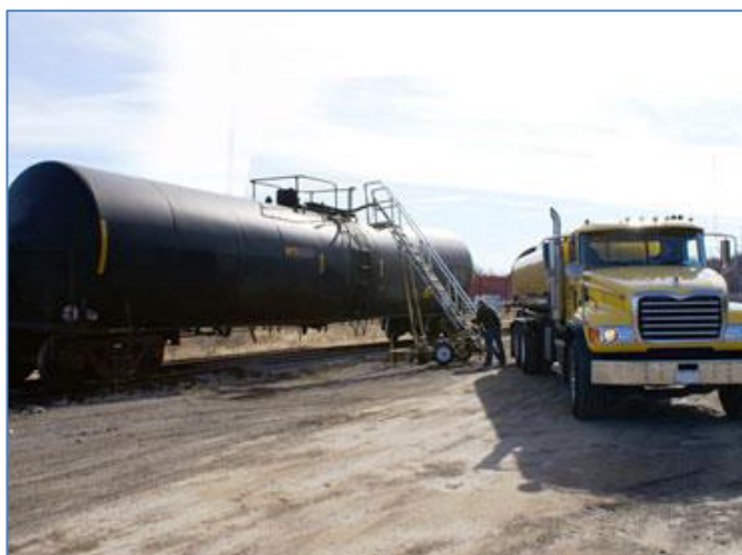
FIGURE 3-11 Direct truck-to-rail transloading.
