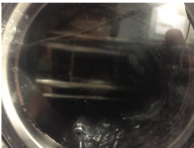
Figure 4.11. Residue from silicone resin evaporated from the paint during baking and left coated onto the front viewport.
