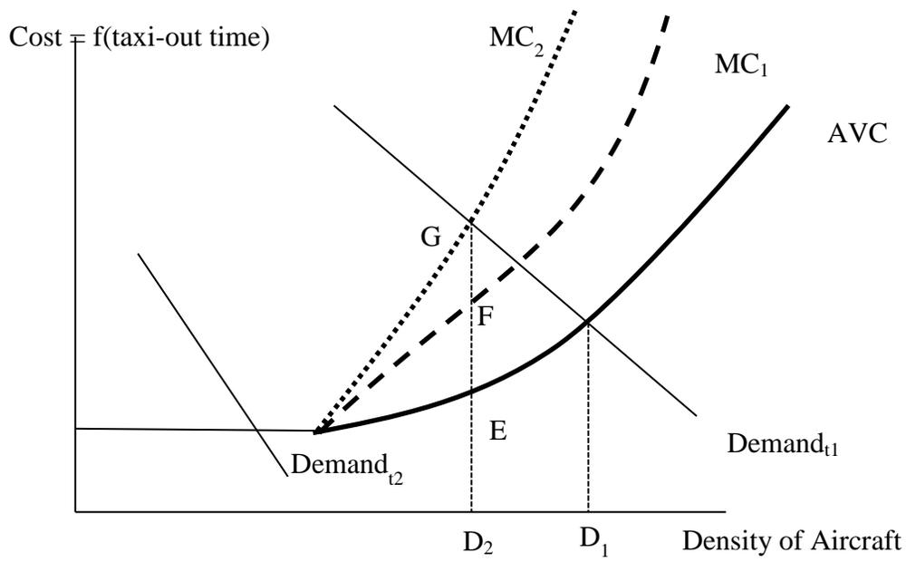
**Figure 1: Standard steady-state congestion model**
