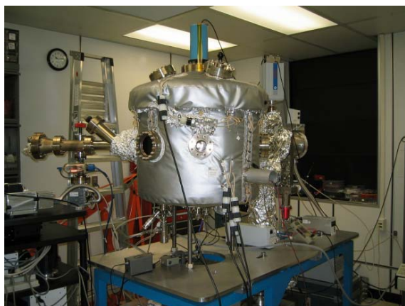
Fig. 1: GSFC UHV photocathode processing chamber
